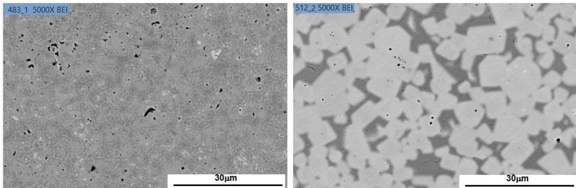
Fig. 11 - Backscattered images for NbC-18Ni-6WC ball milled and for NbC-20Ni-4WC attritor milled pressed (200MPa) and sintered (as Fig. 10) samples.
