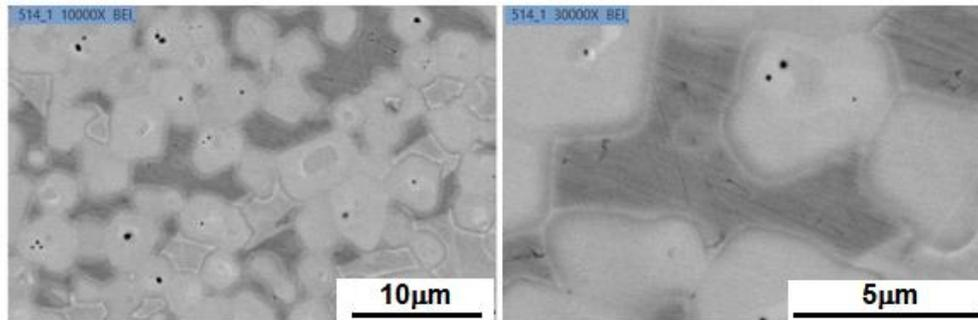
Fig. 15 - Backscattered images for NbC<sub>20</sub>Ni-4WC attritor milled, pressed (50MPa) and sintered in DSC/TG at 1390°C with previous lower temperature (1280°C for 1 hour), sample.
