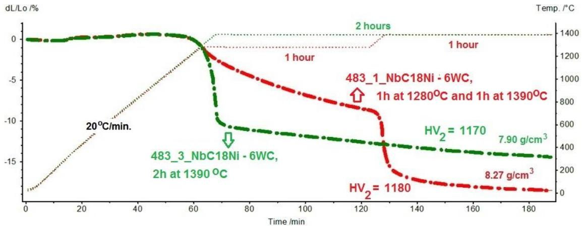
Fig. 6 – Dilatometric curves for NbC-18Ni-6WC ball milled samples pressed at 200MPa. Heating rates of 20°C/min., with (483\_1) and without (483\_3) a lower temperature (1280°C) step. Dynamic argon (200ml/min.) atmosphere.
