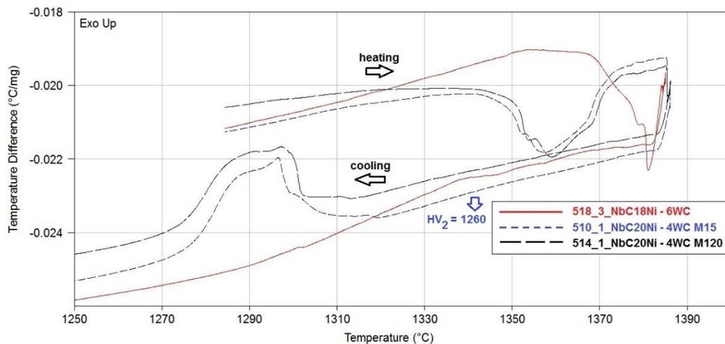
Fig. 5 - DSC curves for NbC-20Ni-4WC attritor milled (15 and 120 min.), and for NbC-18Ni-6WC ball milled, pressed samples. Heating at 20°C/min. up to 1280 °C, 60 min. at 1280 °C, 5°C/min. up to 1390 °C, 60 min. at 1390 °C and colling down at 5°C/min. up to 1200°C. A dynamic atmosphere of nitrogen, 200ml/min., was used.
