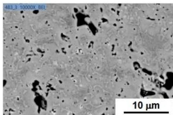
Fig. 8 – Backscattered image of NbC-18Ni-6WC ball milled and pressed (200MPa) sample. One step: 2 hours at 1390°C.
