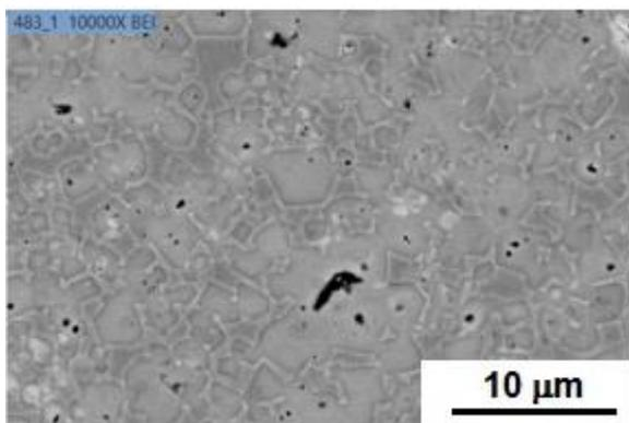
Fig. 7 – Backscattered image of NbC-18Ni-6WC ball milled and pressed (200MPa) sample. Two steps: 1h at 1280°C, and more 1h at 1390°C.
