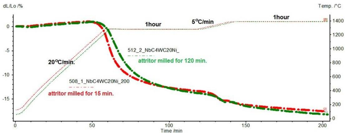
Fig. 12 - Dilatometric curves for NbC-20Ni-4WC attritor milled and pressed (200MPa) samples. Heating rates of 20°C/min., 1 hour at 1390°C and 1 hour at 1280°C. The sample 508\_1 was from powder milled for 15 minutes and the 512\_2 was milled for 120 minutes. A dynamic argon (200ml/min.) atmosphere was used.
