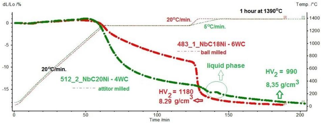
Fig. 10 - Dilatometric curves for NbC-18Ni-6WC ball milled and for NbC20Ni-4WC attritor milled pressed (200MPa) samples. Heating rates and high temperature steps as showed on the figure. A dynamic argon (200ml/min.) atmosphere was used.
