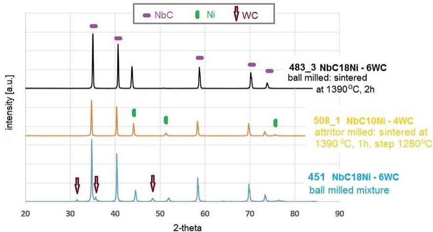
Fig. 9 – DRX for the ball milled mixture and for ball and attritor milled sintered samples. It was used a Cu k- $\alpha$  radiation
