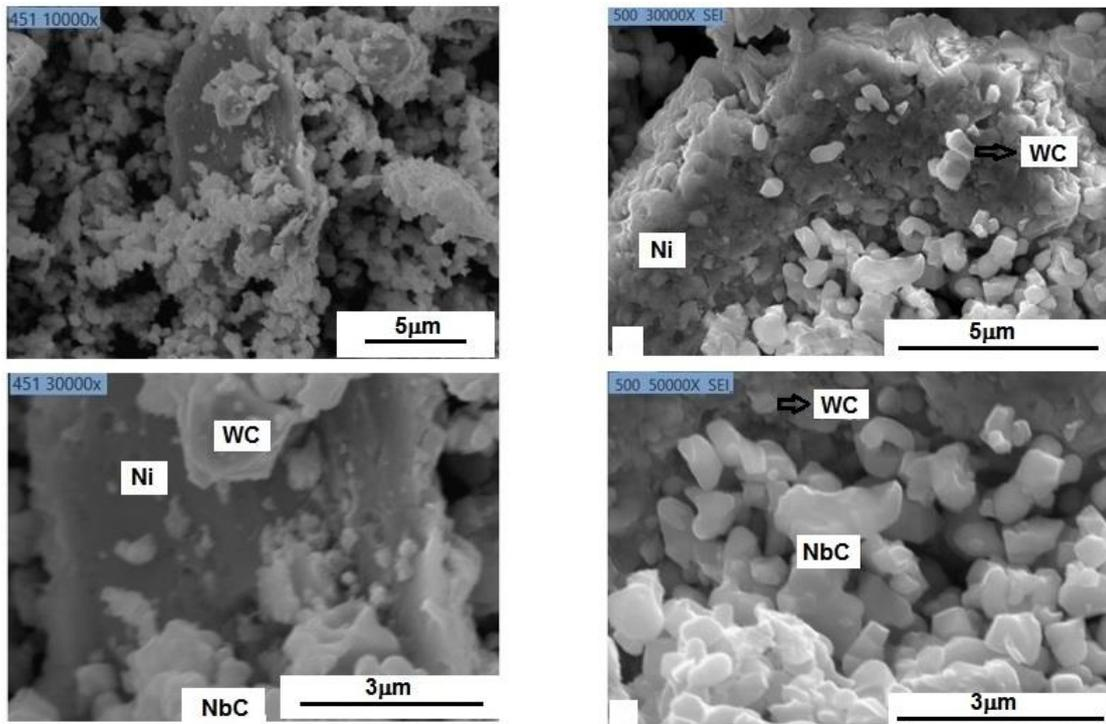
Fig. 2 - The 76wt%NbC, 6%wtWC and 18wt% Ni mixture ball milled for 15 hours. Secondary Electrons Image – SEI.
