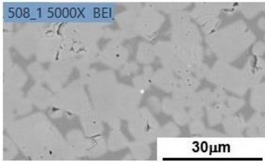
Fig. 13 - Backscattered image for NbC<sub>20</sub>Ni-4WC attritor milled (15 minutes) and pressed (200MPa) sample. Two steps: 1 hour at 1280°C, and more 1 hour at 1390°C.
