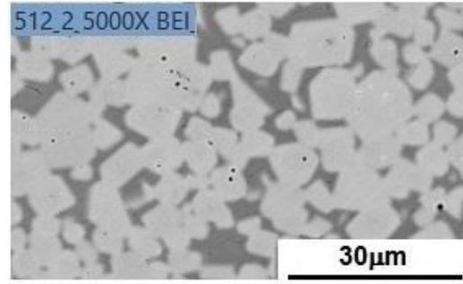
Fig. 14 - Backscattered image for NbC<sub>20</sub>Ni-4WC attritor milled (120 minutes) and pressed (200MPa) sample. Two steps: 1 hour at 1280°C, and more 1 hour at 1390°C.
