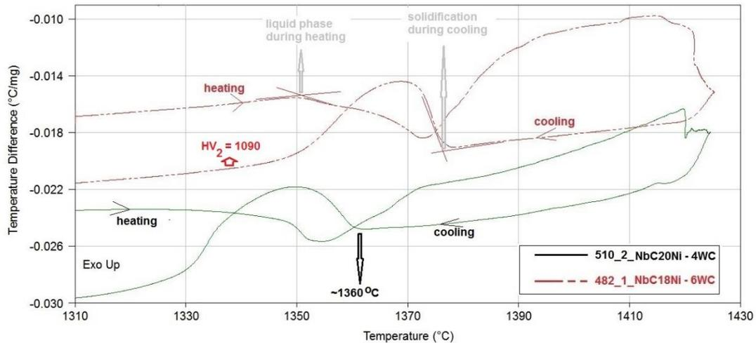
Fig. 4 - DSC curves for NbC-18N-6WC ball milled and NbC-20Ni-4WC attritor milled (15min.), pressed (50MPa) samples. Very quick heating up to 1200°C, heating up at 10°C/min. up to 1430°C, 5 min. at 1430 °C, and cooling down at 10°C/min. up to 1200°C. Dynamic atmosphere of Nitrogen, 200ml/min.
