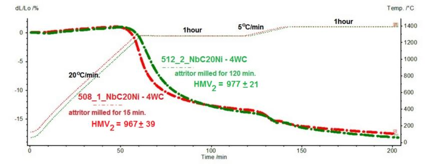
1280 °C, 60 min. at 1280 °C, 5°C/min. up to 1390 °C, 60 min. at 1390 °C and cooling down at 5°C/min. up to 1200°C. A dynamic atmosphere of nitrogen, 200ml/min., was used.
