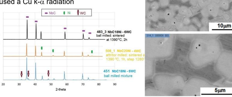
BSI: NbC20Ni-4WC attritor milled, pressed (50MPa) and sintered (1390°C) (DSC/TG) sample. Previous lower temperature (1280°C for 1 hour),.
