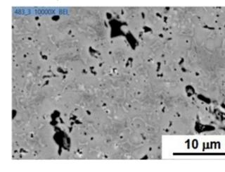
BSI: NbC-18Ni-6WC ball milled and pressed (200MPa) sample. One step: 2 hours at 1390°C.
