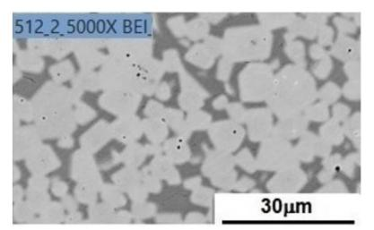
BSI: NbC20Ni-4WC attritor milled (120 minutes) and pressed (200MPa) sample. 1 hour at 1280°C, and more 1 hour at 1390°C.
