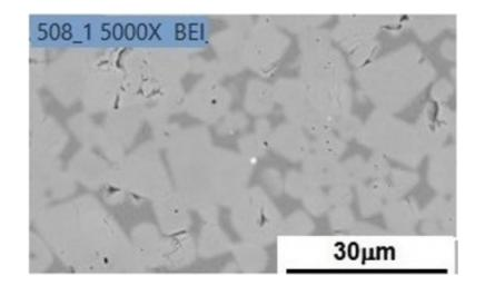
BSI: NbC20Ni-4WC attritor milled (15 minutes) and pressed (200MPa) sample. Two steps: 1 hour at 1280°C, and more 1 hour at 1390°C.
