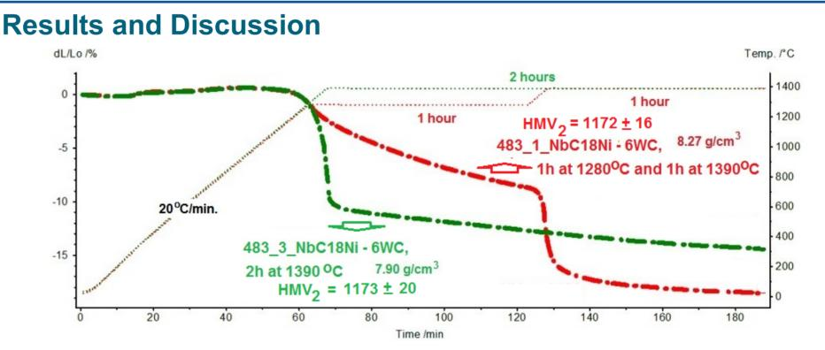
Dilatometric curves for NbC-18Ni-6WC ball milled samples pressed at 200MPa. Heating rates of 20°C/min., with (483\_1) and without (483\_3) a lower temperature (1280°C) step. Dynamic argon (200ml/min.) atmosphere.
