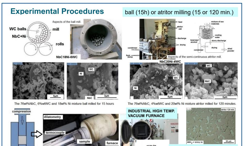
applications. The binder content used here was close to 20wt% and coarse grain size was the goal to be achieved. Densities close to  $8.30g/cm^3$  and Vickers Hardness (HMV<sub>2</sub>) close to 1100 were expected. Two chemical compositions and two milling processes were investigated. The sintering was monitored in a dilatometer and also by thermal analysis. The presence of a liquid phase, the shrinkage and the microstructural aspects are presented and discussed.
