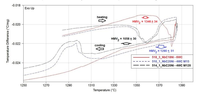
DSC curves for NbC-20Ni-4WC attritor milled (15 and 120 min.), and for NbC-18Ni-6WC ball milled, pressed samples. Heating at 20°C/min. up to
